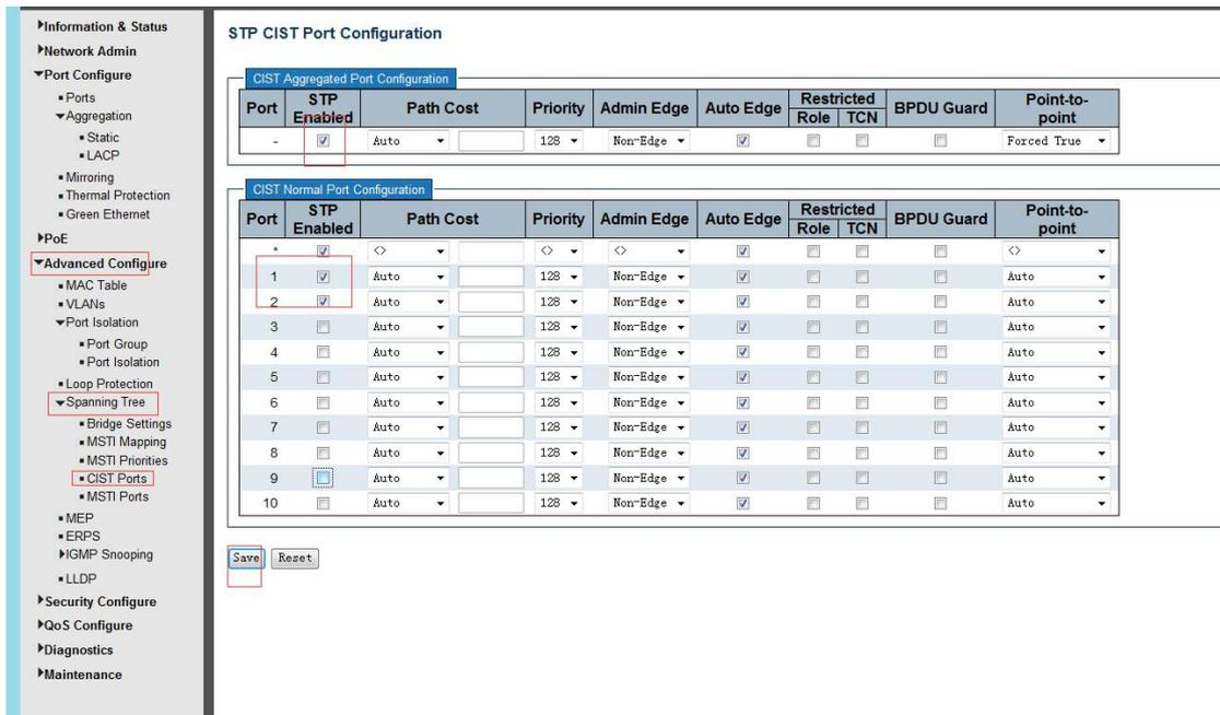
3. Testing configuration result. The port 1 of switch D is blocked. The network structure is tree type.
