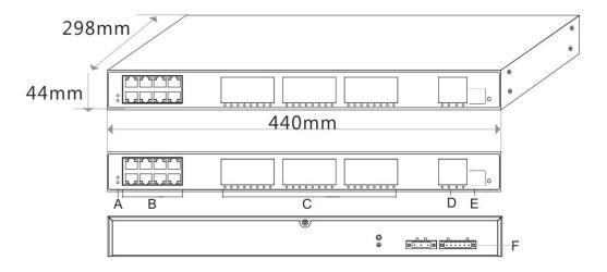
A.Working indicator C. 24\*Gigabit SFP Ports E.Console port B. 8\* RJ45 Ports D.4\*1/10G SFP+ Ports F.AC/DC dual input port
