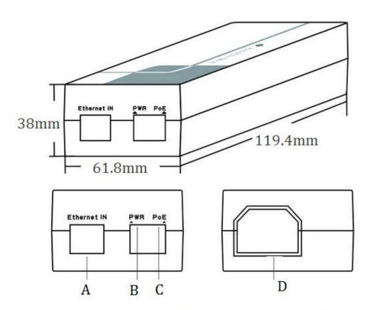
A. Ethernet input RJ45 port B. Working status indicator
