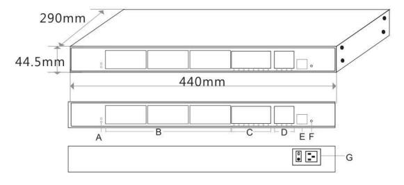
A. Working indicator B. 24\*10/100/1000M RJ45 ports
