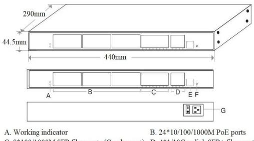
C. 8\*100/1000M SFP fiber ports (Combo port) D. 4\*1/10G uplink SFP+ fiber ports
