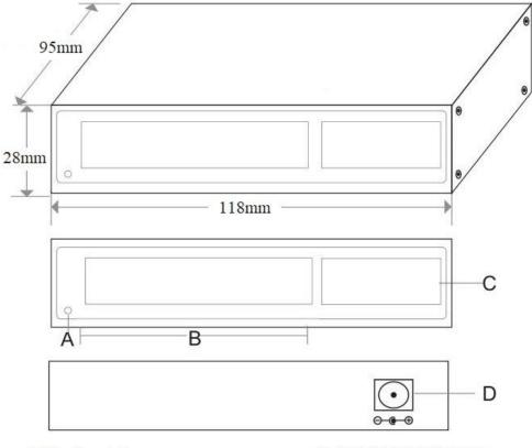
A. Working indicator C. 2\*10/100/1000M uplink RJ45 ports
