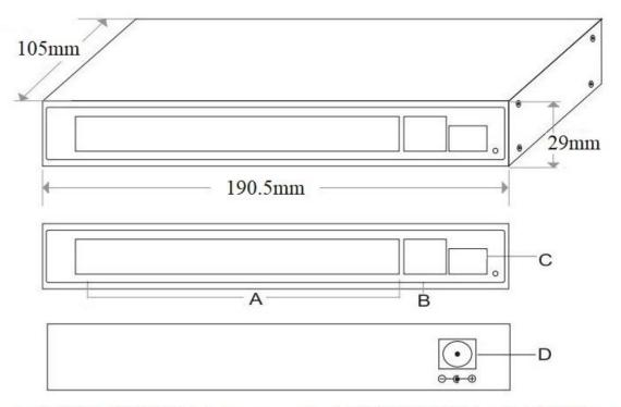
A. 8\*10/100/1000M PoE ports B. 1\*10/100/1000M uplink RJ45 port C. 1\*1000M uplink SFP fiber port D. Power input port DC48-57V
