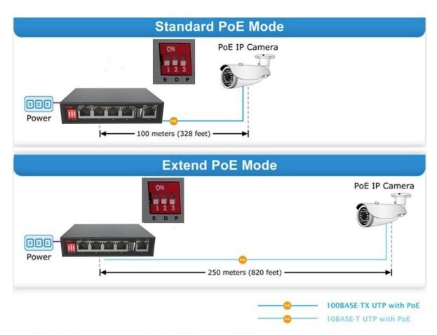
Extend network communication distance and PoE power supply distance.
