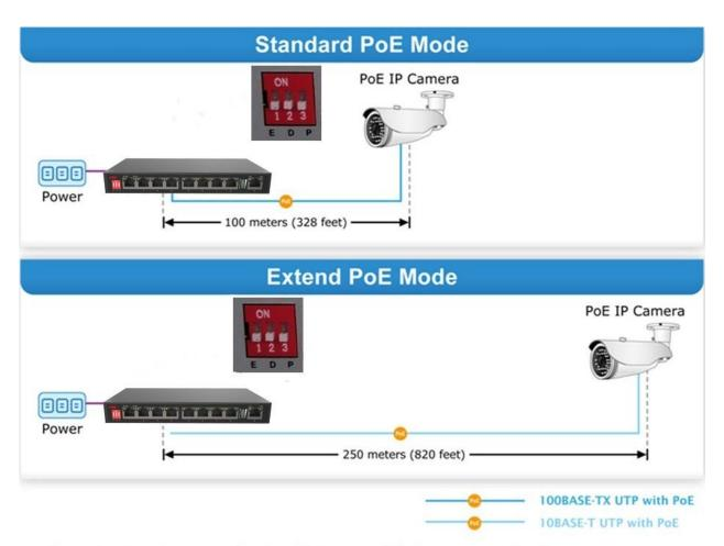
Extend network communication distance and PoE power supply distance.
