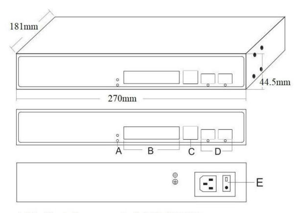
A. Working indicator B. 4\*10/100/1000M RJ45 ports
