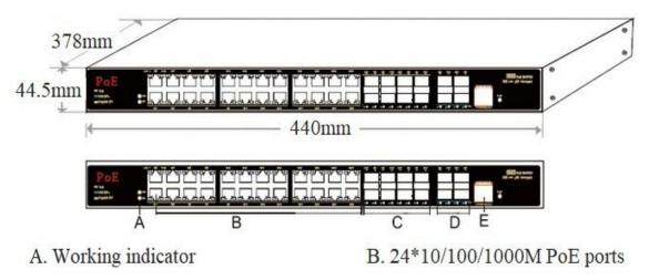
C. 8\*100/1000M uplink SFP fiber ports D. 4\*1/10G uplink SFP+ fiber ports E. Console port
